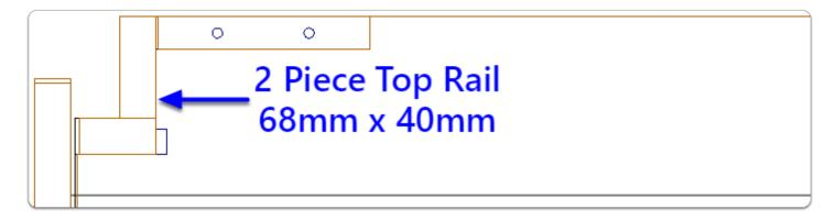
The Cut as One feature shows as 2 rails in the drawing but machines as a single part on the nest. The factory guys can split it up after edge banding.
