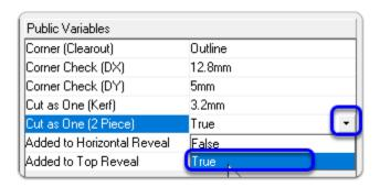
The Cut as One (Kerf) value should match your saw blade thickness...
