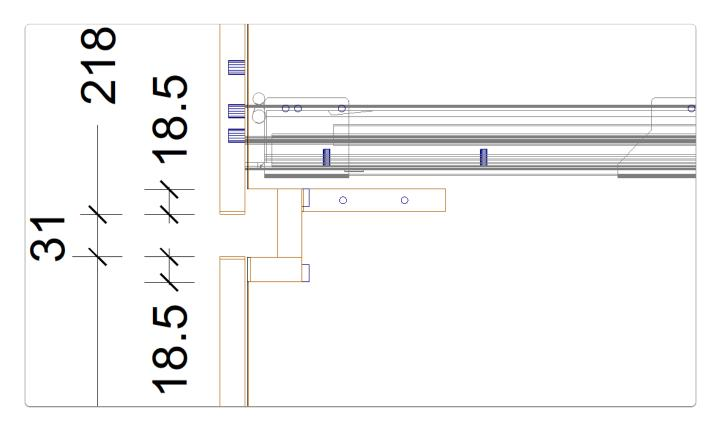
Drawer clearances are automatic, however, the Mid Rail is positioned centrally in height as seen when reviewing the end view above...
