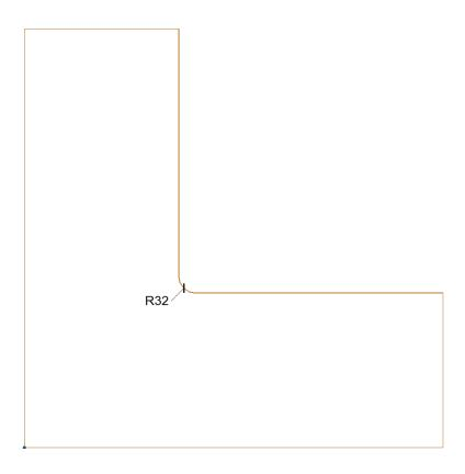
Clipped parts - Top, Deck, Bottom, Shelf, Adjustable Shelf and Fixed Shelf with *rounded* internal corner
